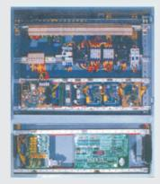
The control panel operates on 440 AC/ 110 DC Volts with Micro processor based down collective system. It is a trouble-free system with maximum efficiency and for longer life. This is fixed in a control box, mounted on either Floor or wall with phase reversal as well as overload protection devices.
