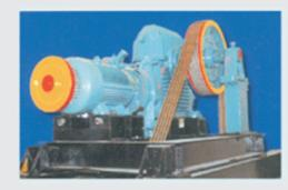
Winding Gear is the worm & worm wheel type, fitted with thrust ball bearing of foreign make. The worm shaft is turned on a single forge of high tensile steel & worm wheel rim of centrifugally cast phosphor bronze, mounted in cast iron dust & leak proof housing to ensure the highest efficiency & noiseless running. Traction sheave & worm wheel are both securely mounted on a substantial steel foundation.
